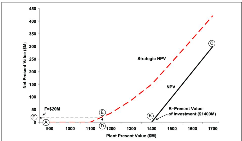
Figure 7 — Intrinsic Value of the Nuclear Plant
